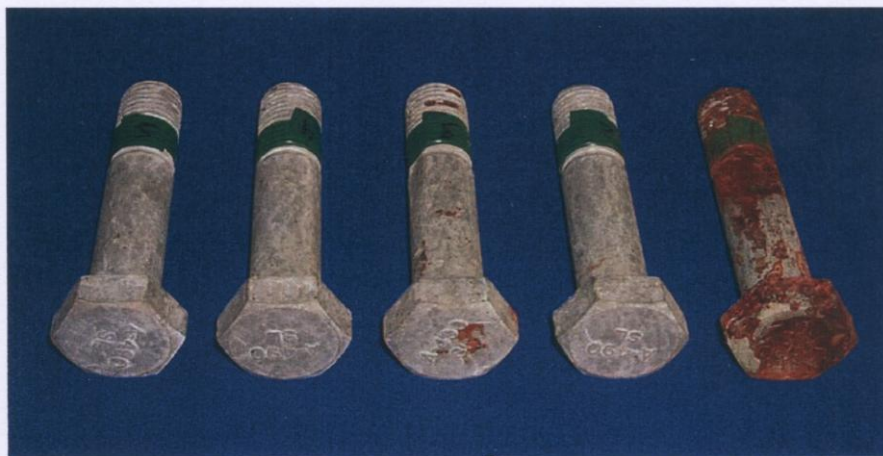
Figure 12: SL std (DACROMET® + 5000 hrs per ASTM B117)
