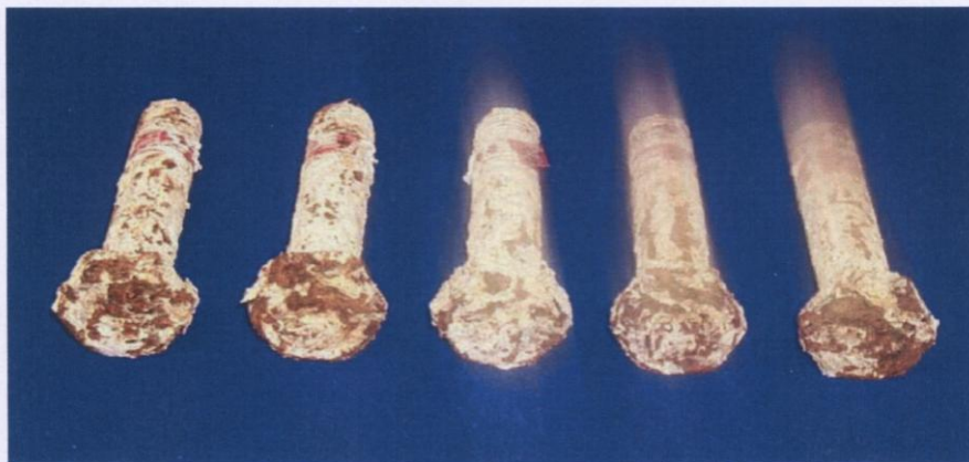
Figure 13: SL std (HDG + 5000 hrs per ASTM B117)
