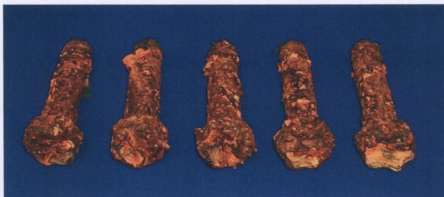
Figure 14: SL std (MG + 5000 hrs per ASTM B117)
